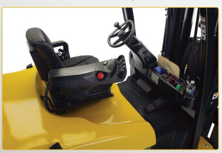
Selecting 'Mode 4' provides maximum speed and acceleration whilst 'Mode 1' is ideal for more precise manoeuvring. Yale trained service technicians can easily adjust the top speed and acceleration.
