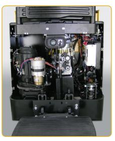
The maintenance free motor (inspection intervals required every 1000 operating hours) provides low cost long operative life. The servo-steering with brushless type DC motor with permanent magnets is maintenance free and incorporates the electronic control system. The DC compound 3kw lifting motor provides power in excess of the truck's operative requirements.
