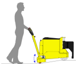
Self-adjusting castor guard for foot protection
