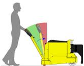
Automatic cut off when tiller arm returns to vertical
