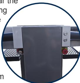
Safety position with double sensor pedal and double hand sensor allow activation of the functions. These safety devices serve to guarantee the stable position of the operator, with both hands on the controls before these become activated.
