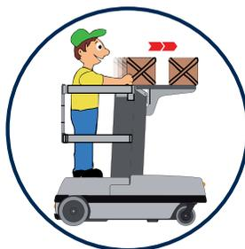
Loading platform at maximum height corresponds to the column. It is very easy to place even heavy packages using the column as the setting base and letting it slide into the material tray
